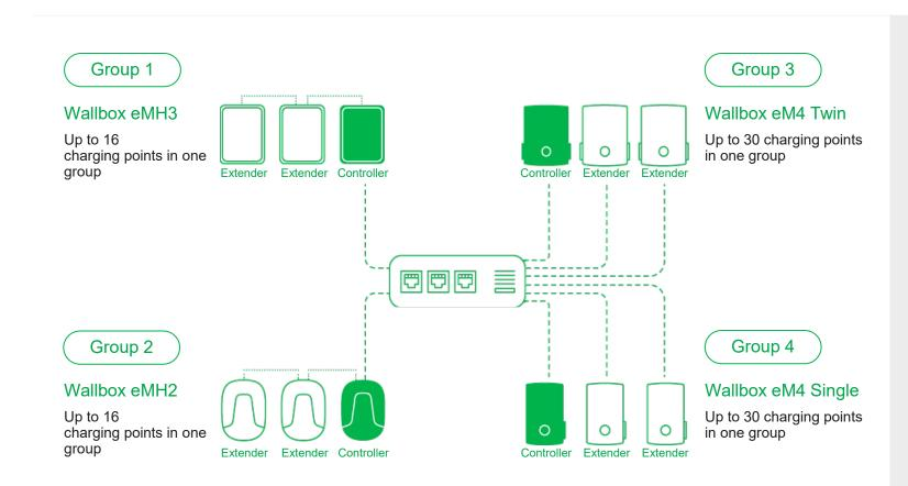
You can expand an existing installation with Wallboxes eM4 Twin or Single. To do this, a Wallbox eM4 Controller must be combined with a controller variant of the Wallbox eMH3 or eMH2 via a router/switch in a multi-group.
